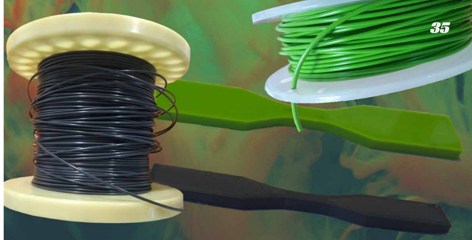
rABS (black) and virgin ABS (green) are processed into filaments. The 3D printed samples are then compared.
